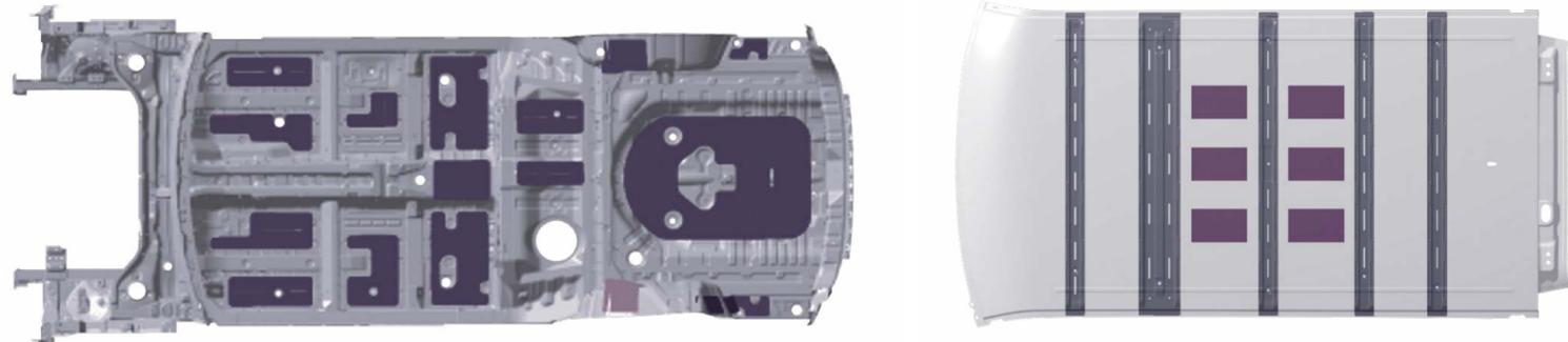
**Underfloor damping and seat/roof panel sound absorbing materials**
