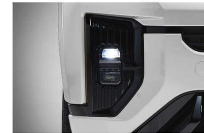
**Automatic headlamps with high beam assist**
