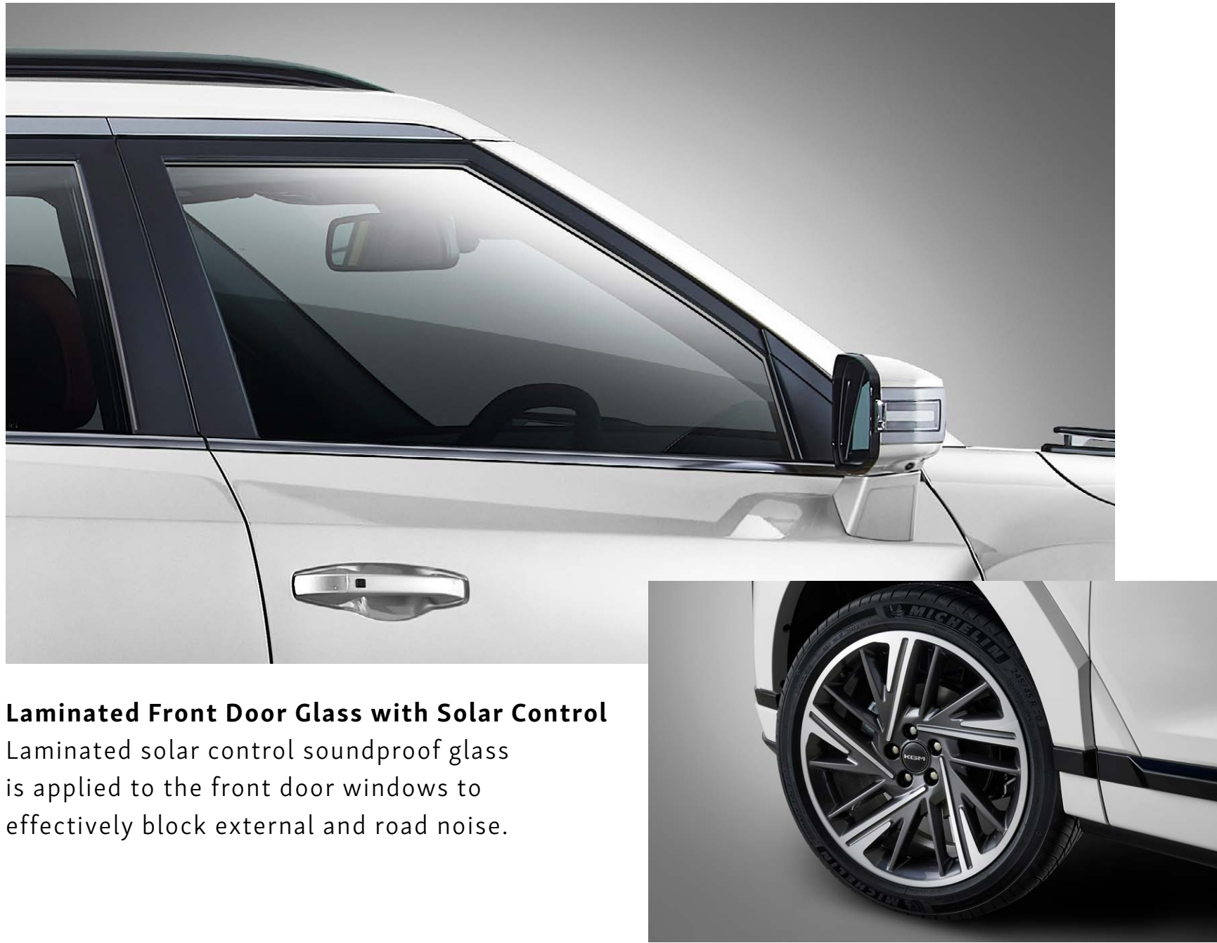
Noise-cancelling Michelin tyres Reduce road noise and tyre resonance by 50%, which is a 10 dB decrease in perceived noise.
