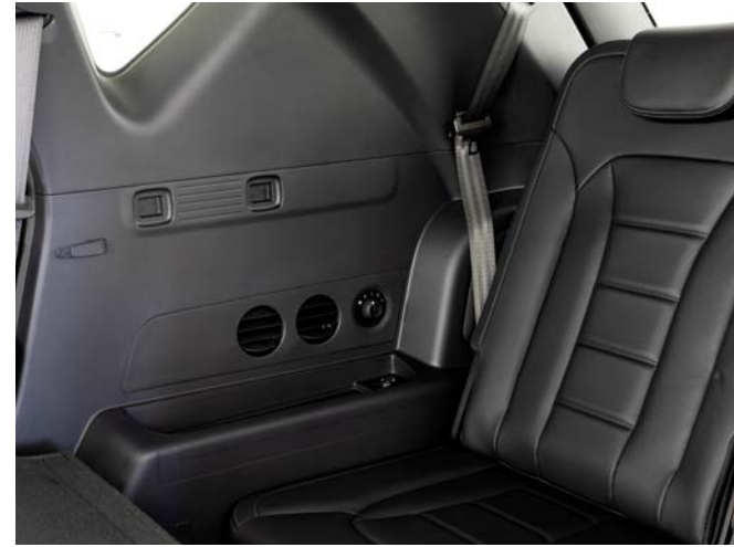
Third row air conditioning
