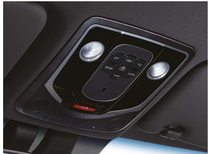
Overhead console with touch-controlled LED cabin lamps
