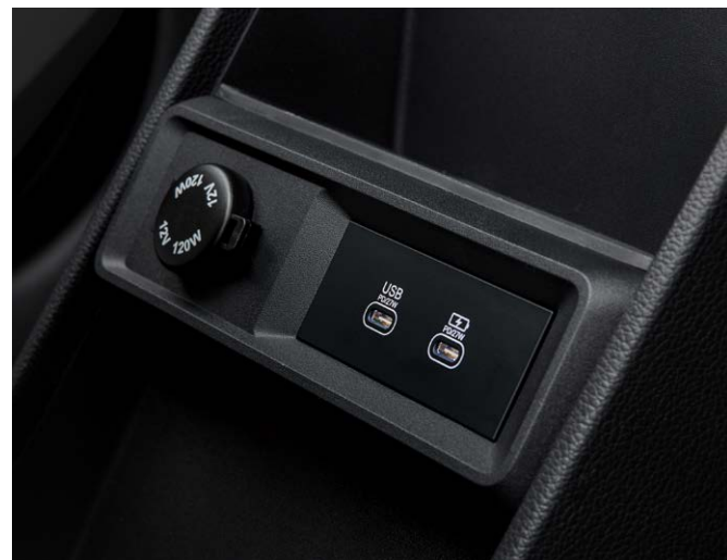
12V power socket in the front, USB charger and USB slot in the rear
