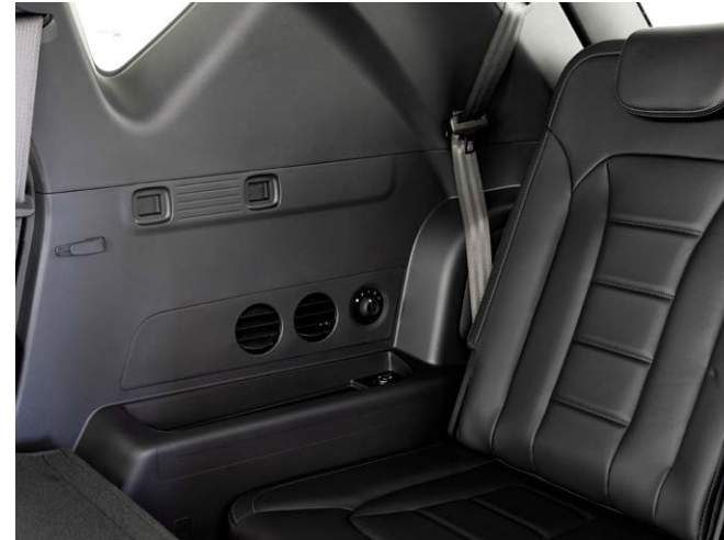
Third row air conditioning
