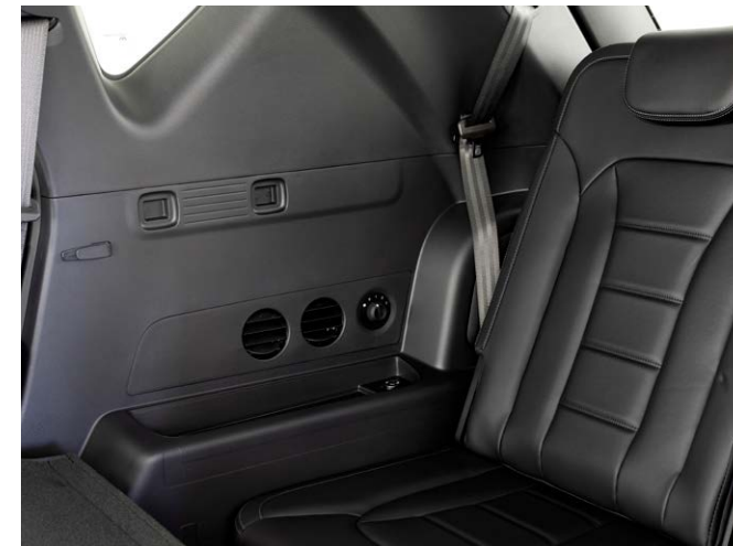
Third row air conditioning
