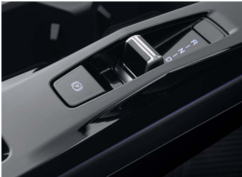
'Shift by wire' toggle switch A 'shift-by-wire" toggle switch replaces the gear shift, making it easier to operate, reduce space, and minimise cabin noise without sacrificing control and convenience.
