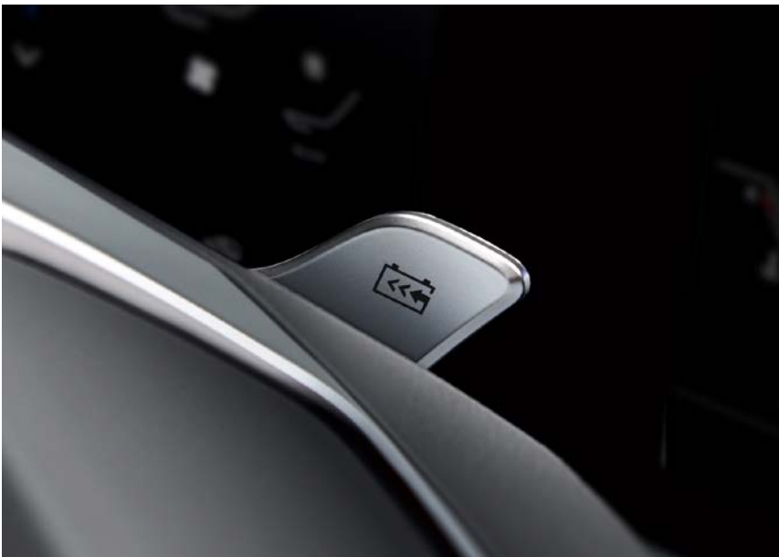
Regenerative Braking System Optimised fuel efficiency is achieved by utilising braking power as battery charging energy.
