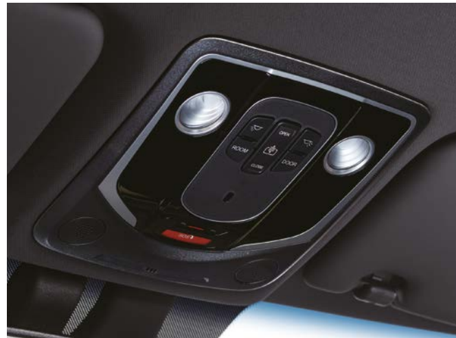
Overhead console with touch-controlled LED cabin lamps
